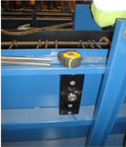
4.1 Placed with magnet in steel form
