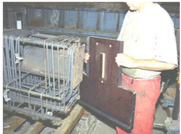
4.4 Endplate with guiding knife Important
