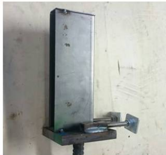
1.4 Column unit with threaded rods and plate washers
