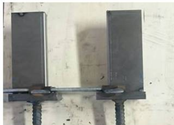
1.6 Column units in pair connected with threaded bar
