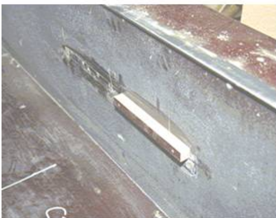
2.5 Guiding knife in right position Important
