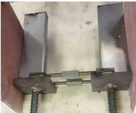
2.3 Shorter bars connected with thread sleeve
