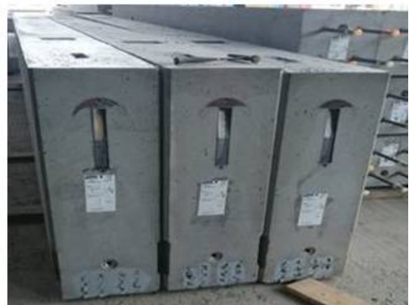
5.6 Finished beams with BSF
