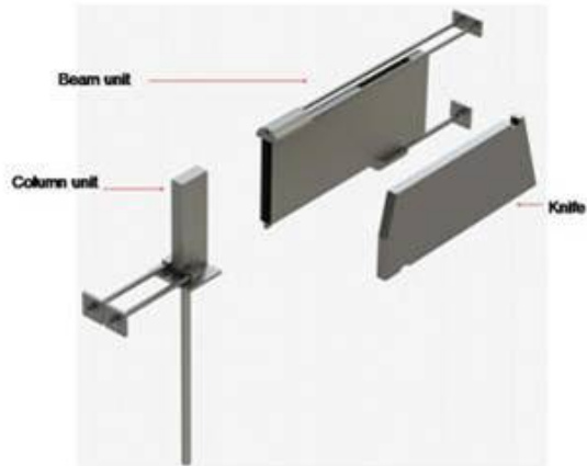
1.1 BSF- , column unit, beam unit and knife
