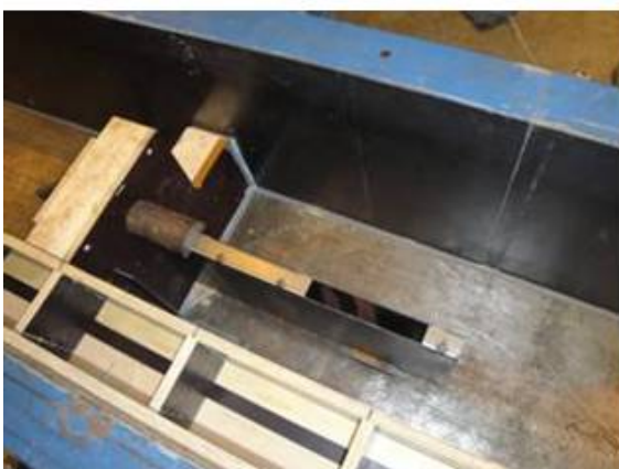
4.5 Endplate with guiding knife Important
