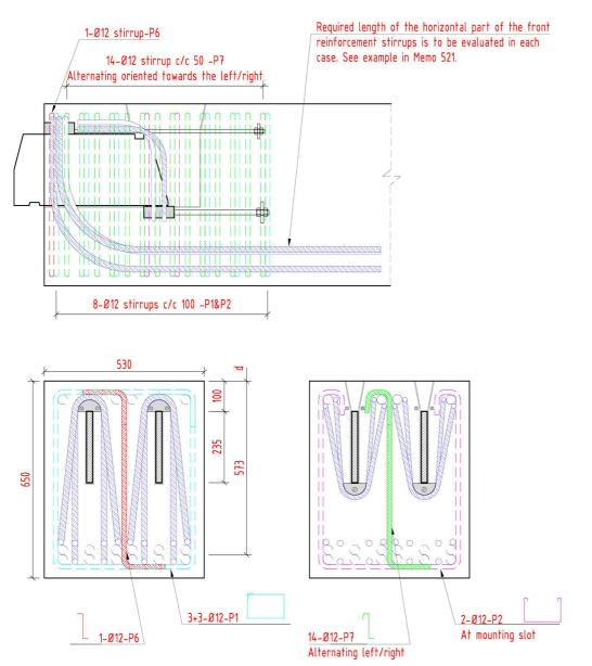
Figure 9: Reinforcement in beam end.
