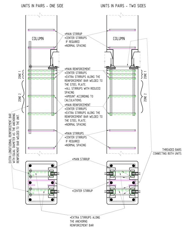
Figure 4: Principal reinforcement in the column.
