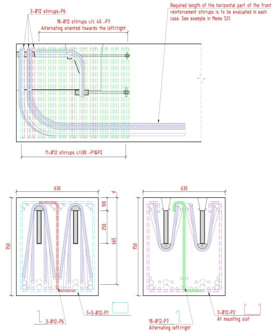
Figure 12: Reinforcement in beam end.
