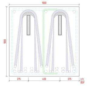
Figure 14: BSF 700 – Recommended minimum cross section and spacing between units when used in pairs.
