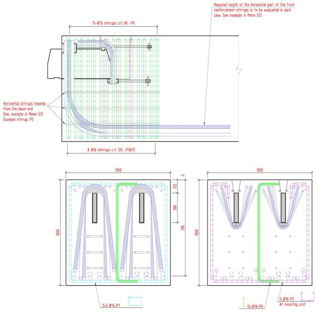
Figure 15: Reinforcement in beam end.
