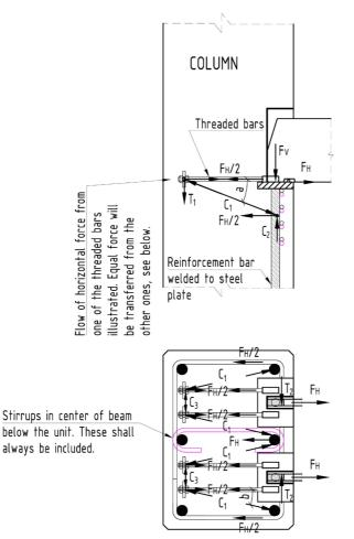
Figure 3: Principal transfer of forces in the column.
