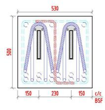
Figure 5: BSF 225 – Recommended minimum cross section and spacing between units when used in pairs.
