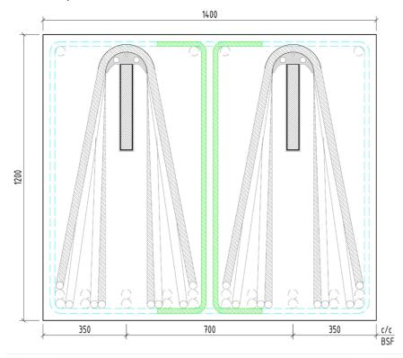
Figure 17: BSF 1100 – Recommended minimum cross section and spacing between units when used in pairs.
