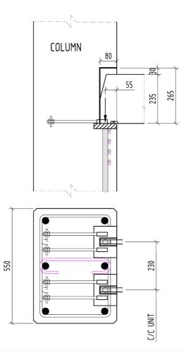
Figure 10: BSF300 column unit. (Reinforcement are not illustrated complete.)
