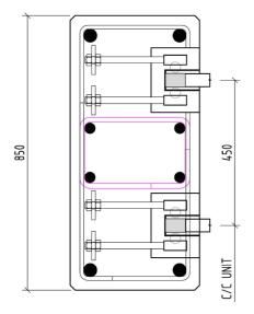
Figure 16: BSF700 column unit. (Reinforcement is not illustrated complete.)
