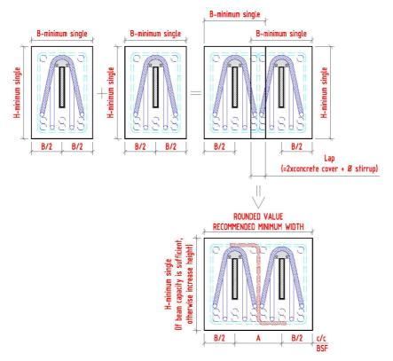
*Figure 1: Principal procedure when defining recommended minimum beam cross-section and distance between units.*
