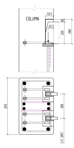
Figure 13: BSF450 column unit. (Reinforcement are not illustrated complete.)
