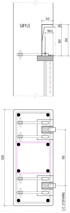
Figure 19: BSF1100 column unit. (Reinforcement is not illustrated complete.)
