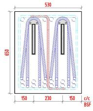
Figure 8: BSF 300 – Recommended minimum cross section and spacing between units when used in pairs.
