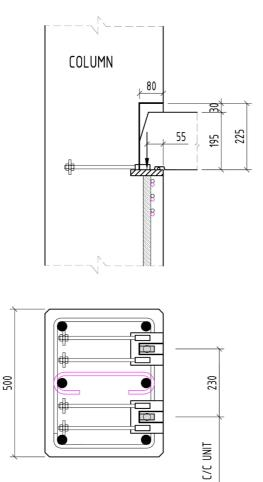
Figure 7: BSF225 column unit. (Reinforcement is not illustrated complete.)
