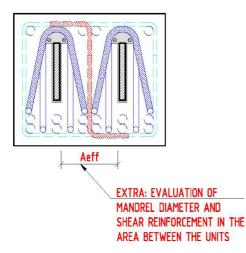
Figure 2: Effective concrete width in-between units.
