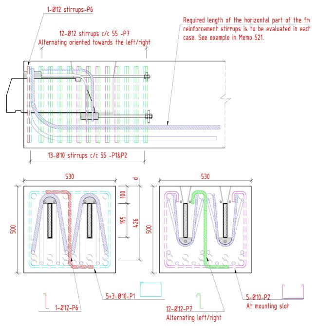
Figure 6: Reinforcement in beam end.
